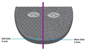
2. If the correct sole was used, then proceed to **ProCover Installation**. Otherwise, replace the old soling using the instructions provided with the replacement soling sheet.
