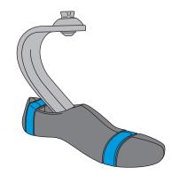
**4.** The cover can be easily removed to aid cleaning the foot and keep the foot in good working order.
